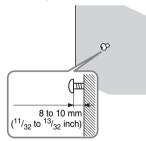
**3** Attach the supplied foot pads to the speakers, and hang the speakers on the screws.
